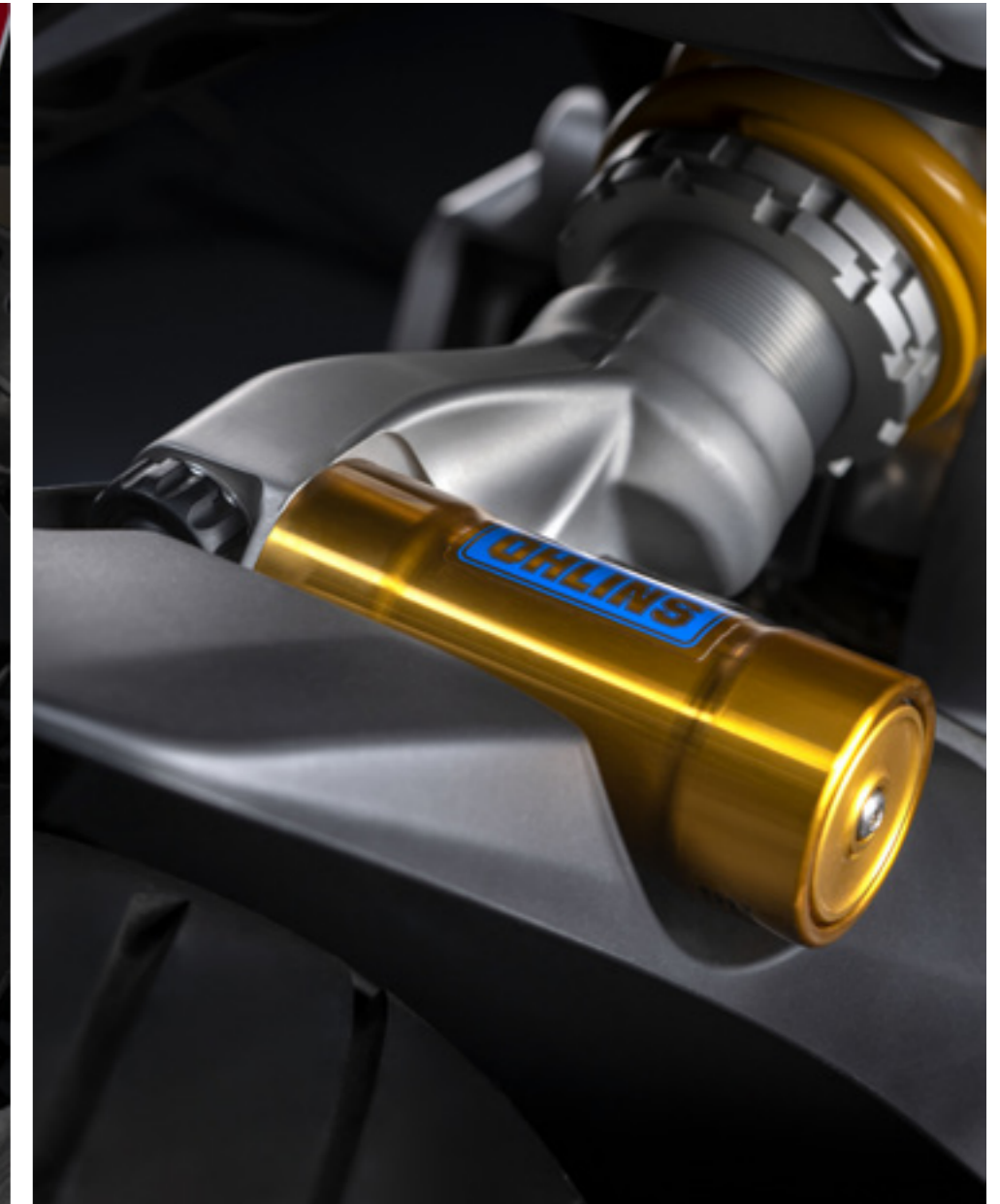
2 Fully adjustable Öhlins monoshock with integrated gas tank.
